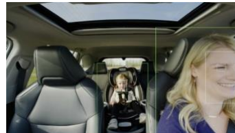
Figure 19 - in-cabin monitoring system
